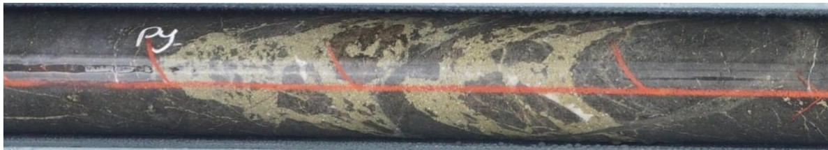
*KSDD050 – A 30cm long pyrite vein breccia within a 1m sample that is grading 28.40g/t Au, 0.02% Cu from 1135m*
